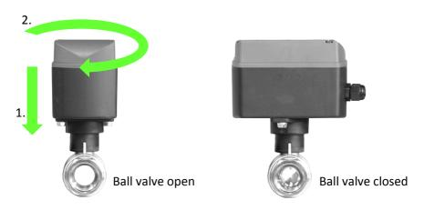
Please note: After a manual override the actuator will be 90° rotated versus the ball valve. All indicators and settings will become reversed, meaning the pre-programmed OPEN and CLOSE settings will become reverse, i.e. OPEN will become CLOSED and CLOSED will become OPEN.
